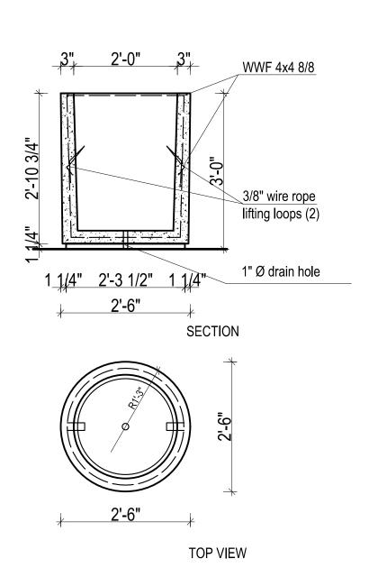
Note: Lifting loops are for plant use and ground movement only and are not engineered for overhead use. Extreme caution must be used when lifting planter from lifting loops higher than 12" from ground.
