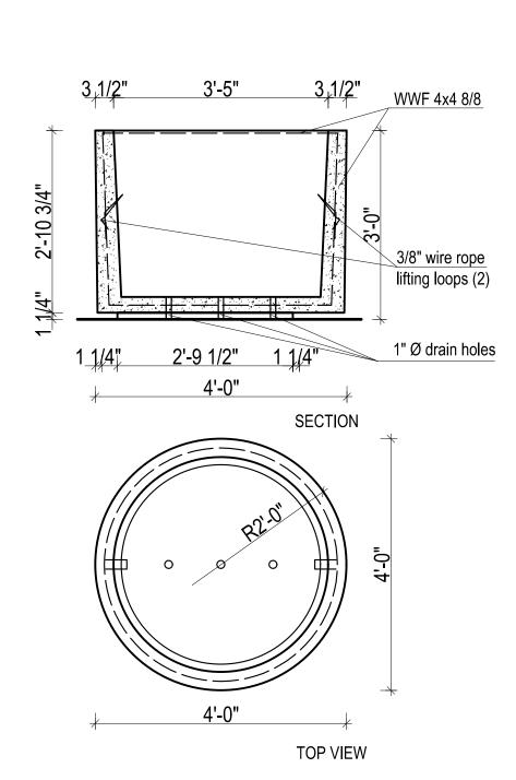
Note: Lifting loops are for plant use and ground movement only and are not engineered for overhead use. Extreme caution must be used when lifting planter from lifting loops higher than 12" from ground.
