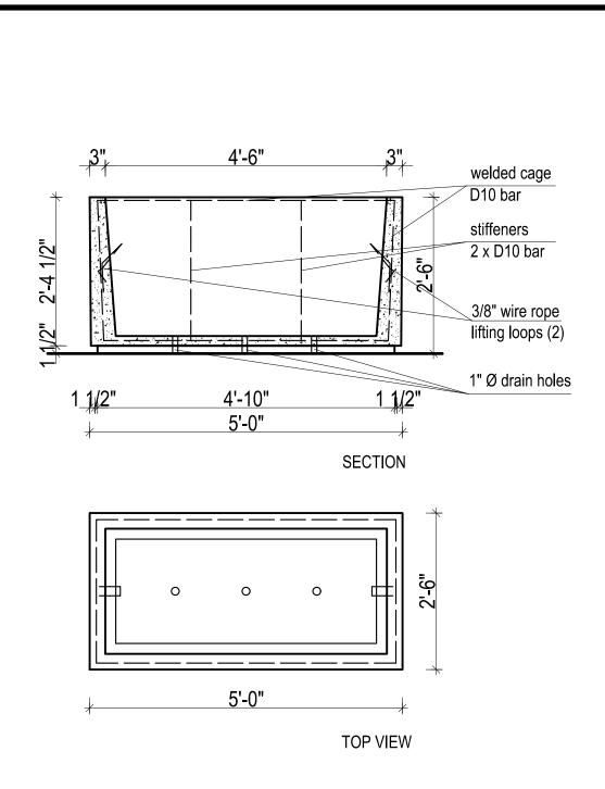
Note: Lifting loops are for plant use and ground movement only and are not engineered for overhead use. Extreme caution must be used when lifting planter from lifting loops higher than 12" from ground.
