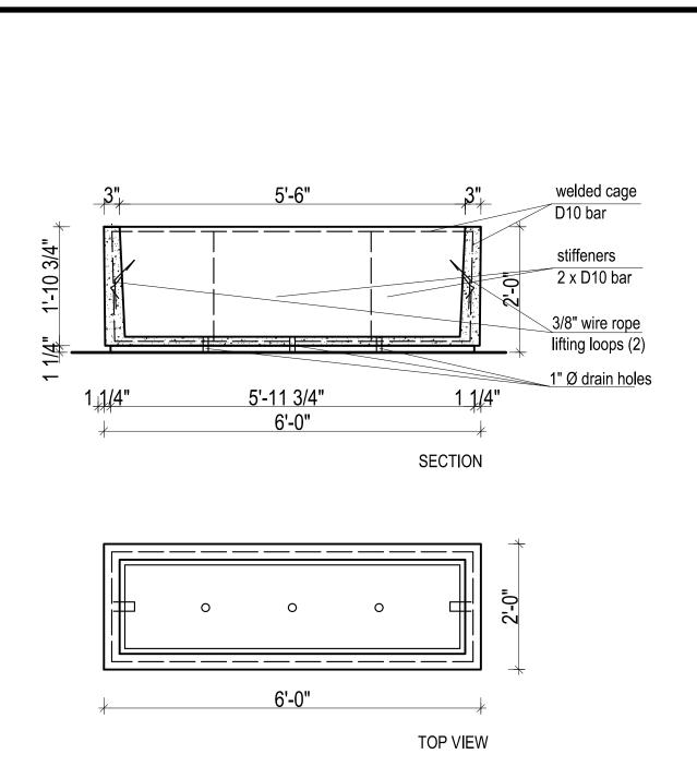
Note: Lifting loops are for plant use and ground movement only and are not engineered for overhead use. Extreme caution must be used when lifting planter from lifting loops higher than 12" from ground.
