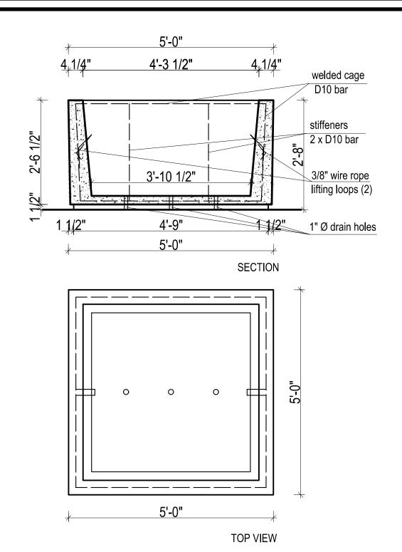
Note: Lifting loops are for plant use and ground movement only and are not engineered for overhead use. Extreme caution must be used when lifting planter from lifting loops higher than 12" from ground.
