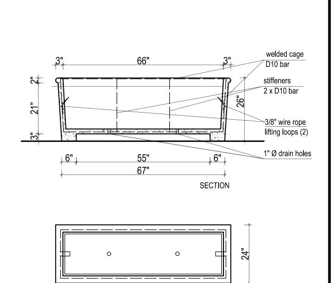
Note: Lifting loops are for plant use and ground movement only and are not engineered for overhead use. Extreme caution must be used when lifting planter from lifting loops higher than 12" from ground.
