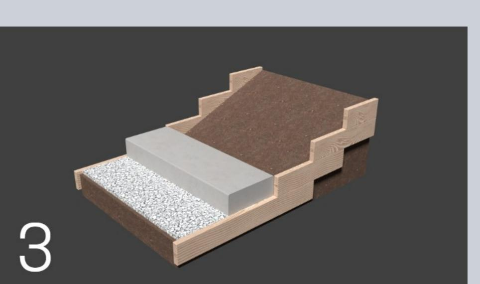
Lay your first Roman step. Check for level and square to the direction on the stairs. The first Roman step is critical as all other steps will follow this initial step. (wood sides not required and are for screed illustration purposes only)
