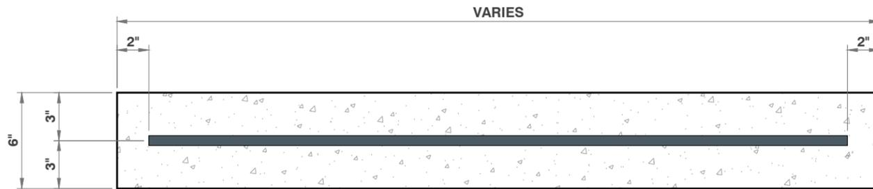
**ELEVATION VIEW REINFORCEMENT**
